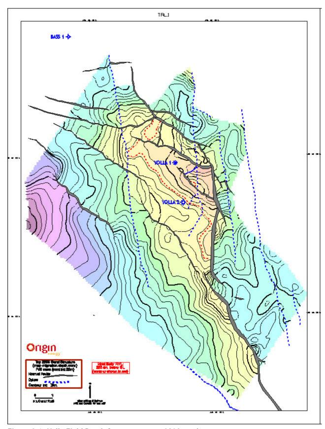
Figure 2.1: Yolla Field Depth Structure at top 2809 sand.
